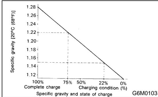
2) Measuring the specific gravity of the electrolyte in the battery will disclose the state of charge of the battery. The relation between the specific gravity and the state of charge is as shown in figure.
