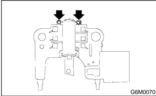
7) Remove the nut and insulating bushing at terminal B, and remove rectifier.
