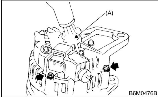
2) Remove the four through bolts. Then insert the tip of a flat-head screwdriver into the gap between the stator core and front bracket. Pry then apart to disassemble.
