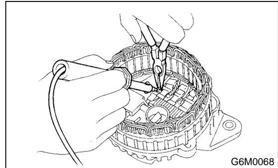
5) Remove screws which secure IC regulator to rear cover, and unsolder connection between IC regulator and rectifier to remove IC regulator.
