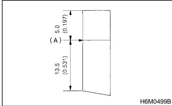
2) Checking brush spring for proper pressure
