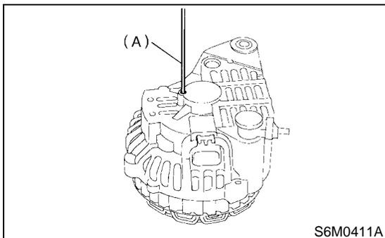
2) Heat the bearing box in the rear bracket [50 to 60°C (122 to 140°F)] and press the rear bearing into the rear bracket.
